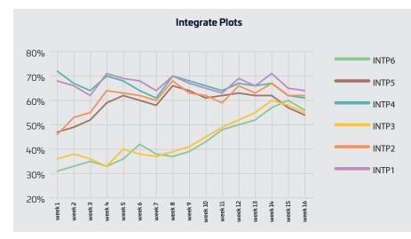
The graph left illustrates the increasing moisture levels which move to almost total homogeneity by week 16.
